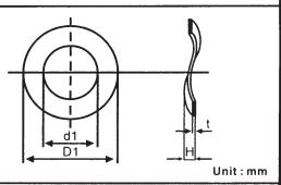
• Material = Carbon spring steel. Hardness HRC 40 to 50, Finish Blue natural Note: 1. Free height H shows when 3 waves are the same height.
